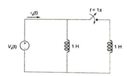
The source voltage  $V_s(t) = \cos(t) \text{ V for } t \ge 0$  and 0 otherwise. The input current  $i_s(t)$  for  $t \ge 0$  is
