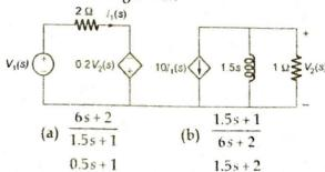
Q.19 For the two port network given below, the value of  $Z_{12}$  is
